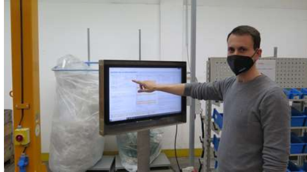
After scanning the barcode, the entire configuration of the bed is visible on the monitor.
