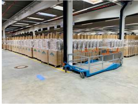
A transport trolley specially developed for Burmeier is pulled to the loading stations by industrial forklifts.
