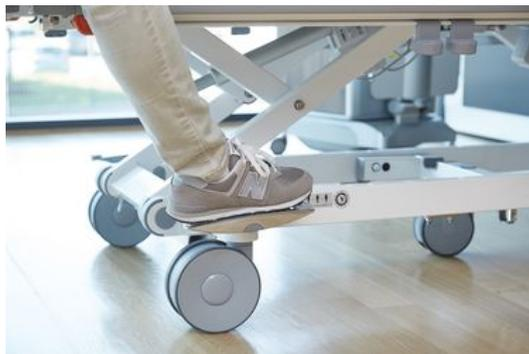
3. To securely steer the bed straight, we recommend activating the directional travel function. To do this, press down on any brake pedal in the direction of the head of the bed.
